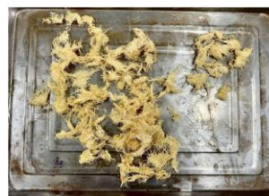
Fig. 2 Cellulose extraction from corn husk
