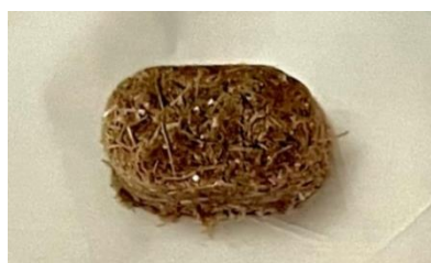
Fig. 1 Biofertilizers pellets prepared from eggshell, chitosan, and rice straw
