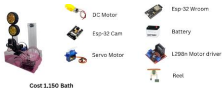
Fig. 3 D-TRACK Cable-Based Robotic Prototype
